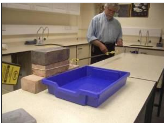
Brickquake, pulled by a winding mechanism © ESEU
